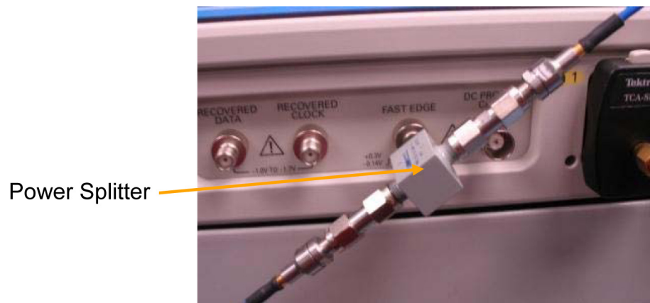
Figure 14: Cable de-skew connections
