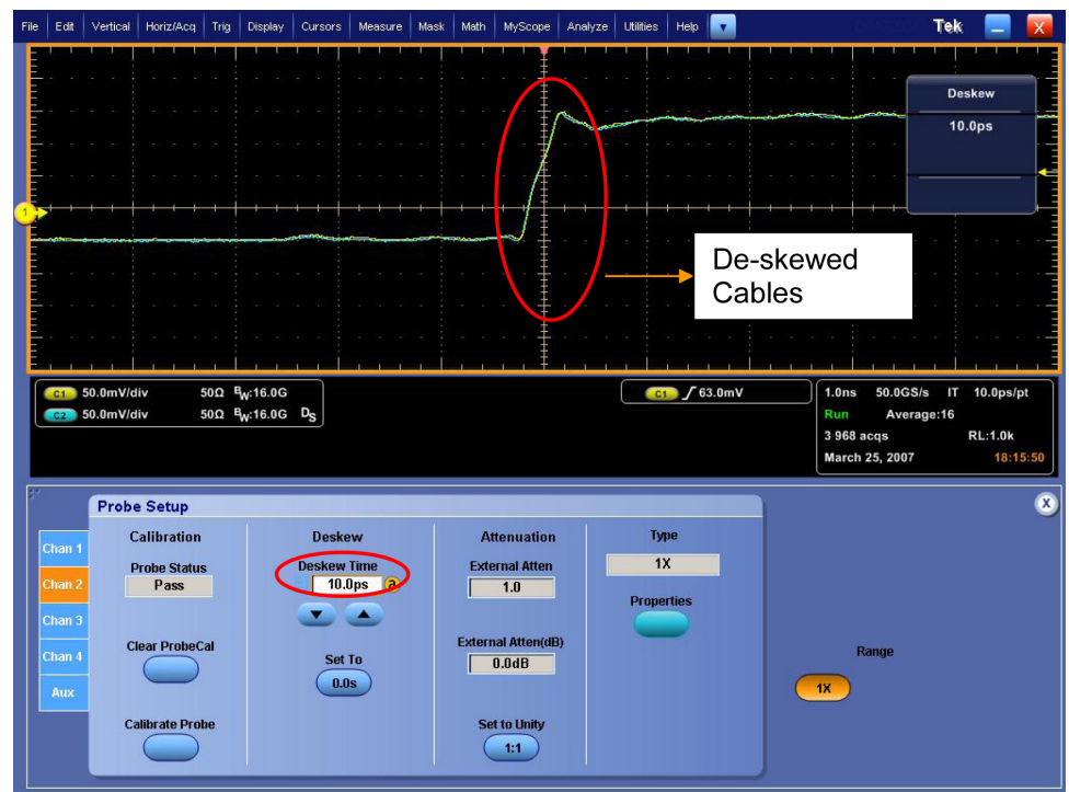
Figure 17: Cable skew adjusted
